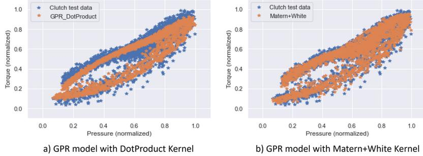
Figure 6: Comparison of wet clutch transfer function built with different kernels
