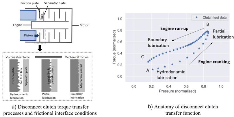
Figure 1: Introduction of wet clutch behavior
