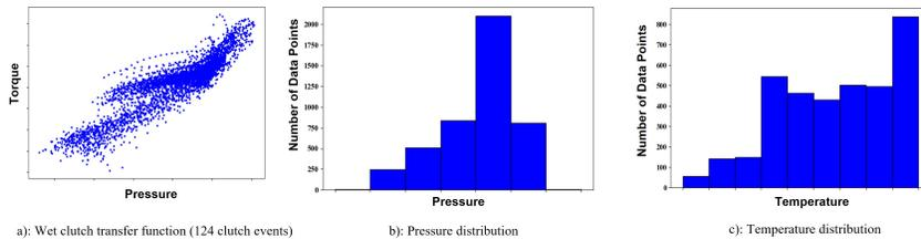
Figure 3: Wet clutch data and its pressure, temperature distribution
