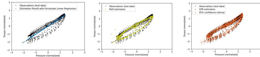
Figure 4: Comparison of wet clutch transfer function built by different ML methods
